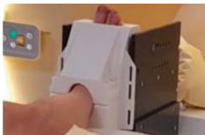
Figure 1: MR-compatible compression device in the MR experiment.
