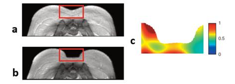
**Results:** The voxel-wise ratios of the out-of-plane displacement to in-plane displacement were higher than 0.5 for more than half of the voxels in the region of indentation for all investigated load cases. This ratio was also equal to or higher than 1.0 for almost half of the voxels in the region for load cases 2-4.
