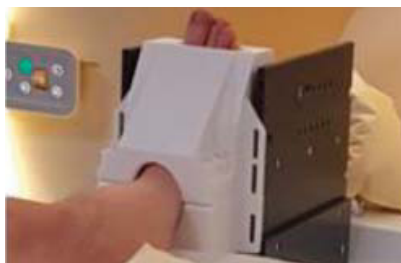
Figure 1: MR-compatible compression device in the MR experiment.
